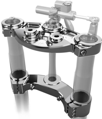
Human Design Weight: 3 kg Safety factor: 2.7 Cost: $
