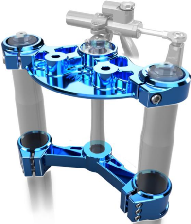
2.5 Axis Generative Weight: 2.3 kg (-23%) Safety factor: 2.2 Cost: $
